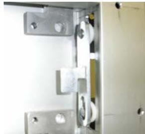
Insert activating assembly, active side first, into muntin channel. Be sure to capture the traveler over the crank. The crank bracket mounting screw should seat into the mounting clips on the active side to assure proper spacing.
