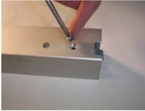
Install top latch mechanism using 2 ea. #10-32x1/4" screws.
